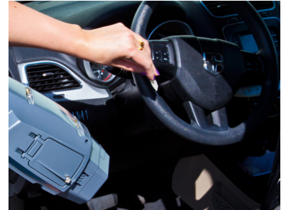
DETECTRA™ HX swipe sampling system is used for advanced detection scenarios.
